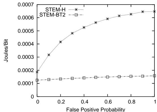
Fig. 12. Energy consumption of STEM-H and STEM-BT2 with false positives.
