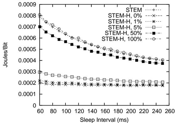
Fig. 10. Energy consumption of STEM and STEM-H with false positives.
