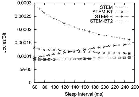
Fig. 9. Energy consumption of the protocols at a higher rate.
