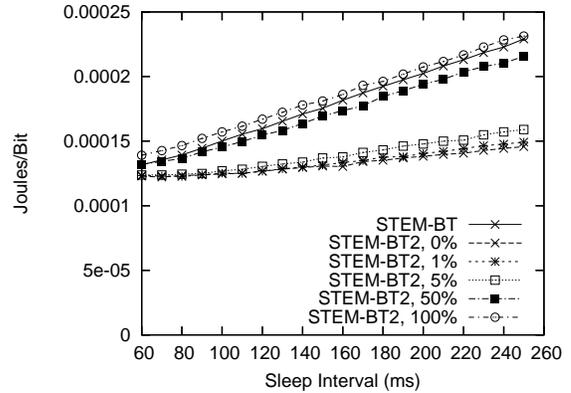
Fig. 11. Energy consumption of STEM-BT and STEM-BT2 with false positives.
