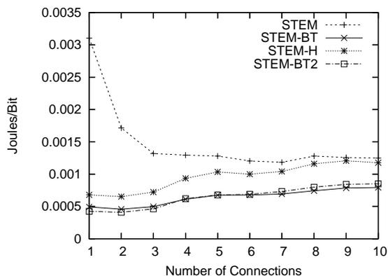
Fig. 13. Energy consumption of protocols in multi-hop scenarios ( $T_{ws} = 100$  ms).
