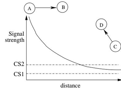
Fig. 2. Larger carrier sense threshold leads to smaller contending area
