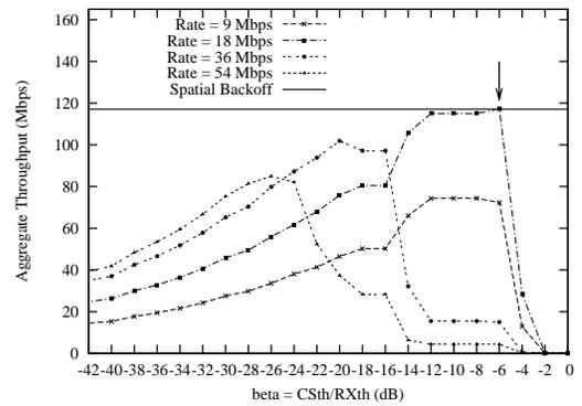
Fig. 3. Aggregate throughput for a circular topology with 32 transmitters
