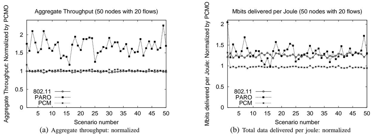
Fig. 10. Random topology for 50 different scenarios with a 25 Kbps data rate per flow (50 nodes in  $1000 \times 1000m^2$ ): 20 flows.
