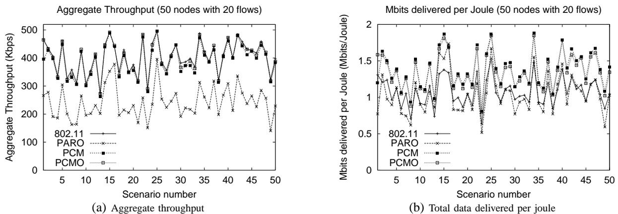
Fig. 9. Random topology for 50 different scenarios with a 25 Kbps data rate per flow (50 nodes in  $1000 \times 1000m^2$ ): 20 flows.
