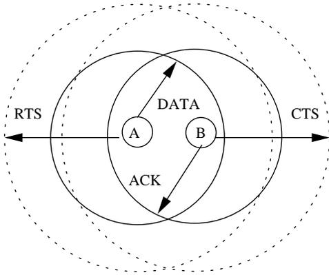
Fig. 1. BASIC: RTS and CTS are transmitted at the highest transmit power, and DATA and ACK are transmitted at the minimum transmit power.
