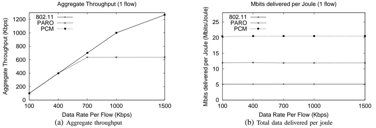
Fig. 3. Chain topology: the curves for PCM+SPR and 802.11 overlap in (a). The aggregate throughput of PARO does not increase beyond 600Kbps due to the contention between two flows.
