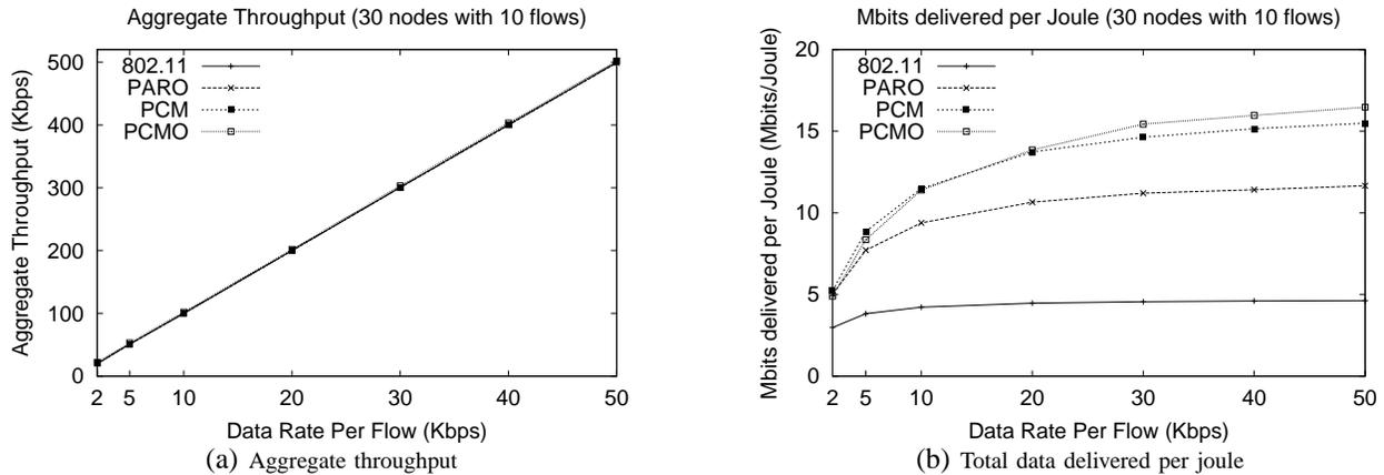
Fig. 4. Random topology with different network loads (30 nodes in  $100 \times 100m^2$ ): the curves for PCM+SPR, PARO, and 802.11 overlap in (a).
