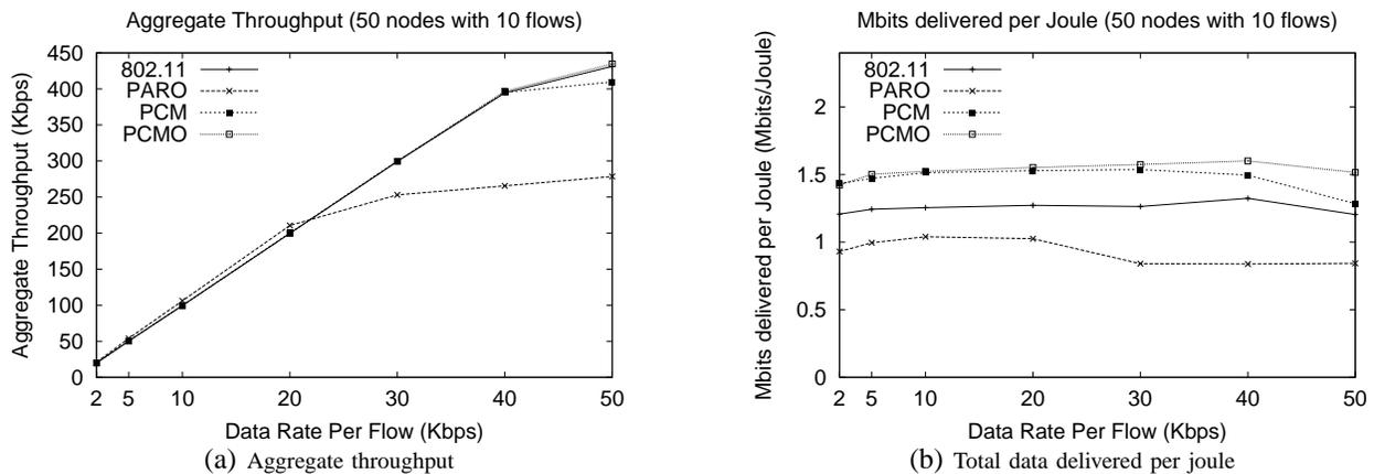
Fig. 5. Random topology with different network loads (50 nodes with 10 flows in  $1000 \times 1000m^2$ ).
