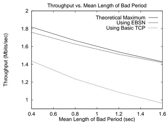
Figure 11: Basic TCP vs EBSN(Local-Area): Mean Good Period=4 sec
