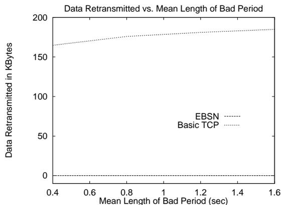
Figure 12: Basic TCP vs EBSN(Local-Area): 4 Mbyte File, Mean Good Period=4 sec
