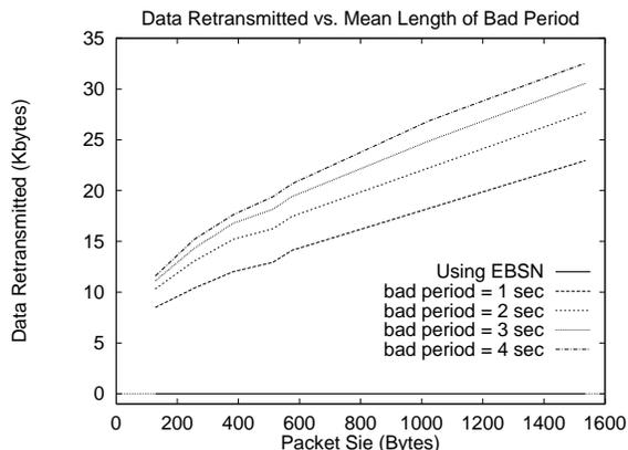
Figure 10: Basic TCP vs EBSN(Wide-Area): 100 Kbyte File, Mean Good Period=10 sec
