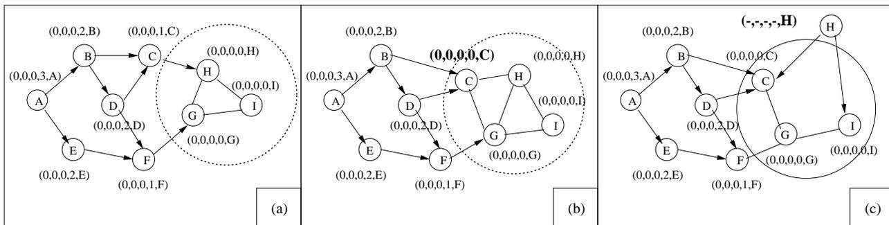
Figure 7: Route Maintenance in GeoTORA for handling dynamic change of geocast group
