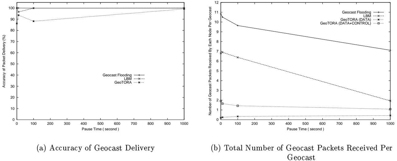
Figure 8: Comparison of GeoTORA to geocast flooding and LBM protocols with a variation of pause time (For 30 nodes, and Maximum speed 5.0 units/sec) : (a) Delivery accuracy versus Pause Time, (b) Total number of packets received per geocast versus Pause Time
