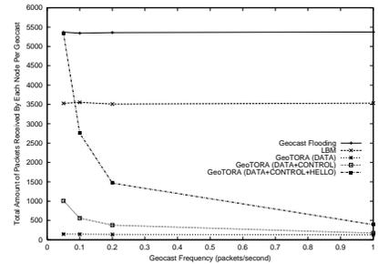
(c) Total Amount of Geocast Packet Received Per Geocast
