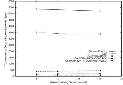
(c) Total Amount of Geocast Packets Received Per Geocast
