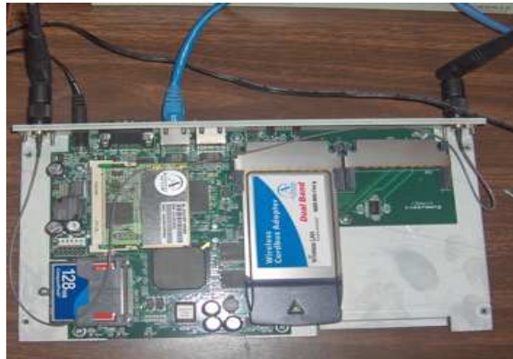
Figure 7.8: Picture of a testbed node. Each testbed node is equipped with two wireless interfaces.
